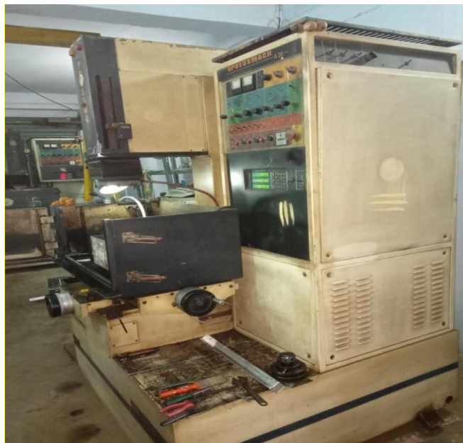
Figure 1 Electrical Discharge Machine experimental set up
